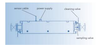
UV monitoring and control by highly selective, calibrated UV sensor
