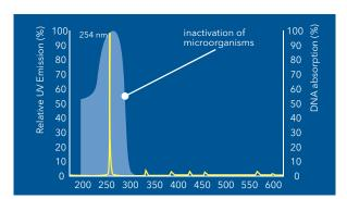
The monochromatic Spektrotherm UV lamp emits at a wavelength of 254 nm, which is in the maximum of the effective disinfection range of the spectrum.
